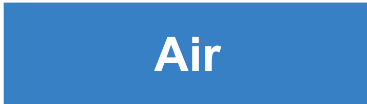
Figure 1 — Example of content name “Air” in the contrast colour white on the basic identification colour blue
