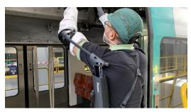
RATP maintenance staff at the Porte des Lilas bus depot are now working with exoskeletons. This innovation is also being trialled by maintenance staff on RER line A and is a great help to operators in carrying out their work. Slipped over the shoulders like a bionic vest, the exoskeleton increases the wearer's physical capacities and reduces strain on the shoulders.
