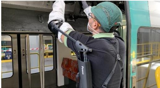
RATP maintenance staff at the Porte des Lilas bus depot are now working with exoskeletons. This innovation is also being trialled by maintenance staff on RER line A and is a great help to operators in carrying out their work. Slipped over the shoulders like a bionic vest, the exoskeleton increases the wearer's physical capacities and reduces strain on the shoulders.
