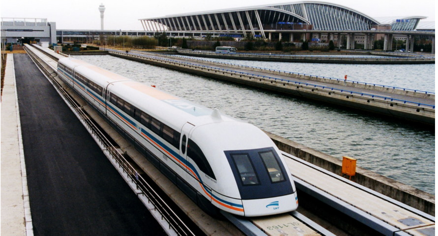
Image 1. A maglev train brings passengers out of the Pudong International Airport in Shanghai, China. Maglev trains are powered by electromagnets. Photo by: Alex Needham via Wikimedia Commons
