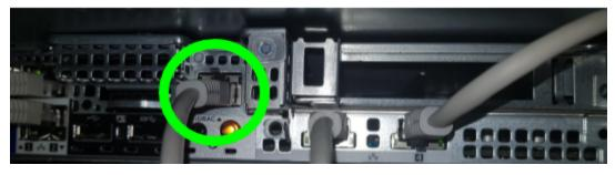
The IPMI interface will acquire a network address over DHCP.
