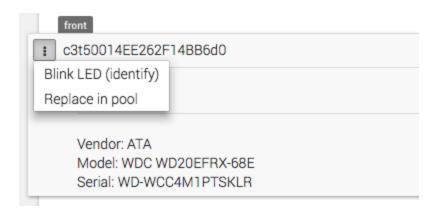
Go to the physical machine. Identify the faulted disk, take the bay out. Replace the disk in the bay with a new disk.
