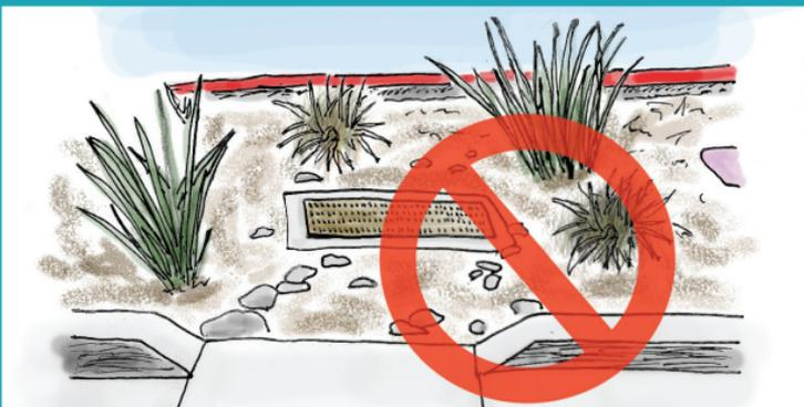
When not properly elevated, runoff merely goes "down the drain." If you are designing or constructing a stormwater landscape, make sure that overflow units are set at the proper elevation.
