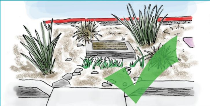
Raised overflow units are often used to help keep stormwater in the landscaped area so it can infiltrate naturally into the soil.
