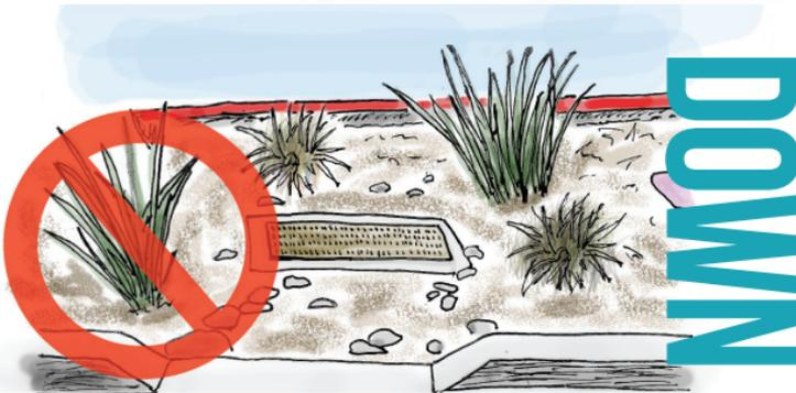
When not properly elevated, runoff merely goes "down the drain." When designing or constructing a stormwater landscape, make sure overflows are set at the proper elevation.
