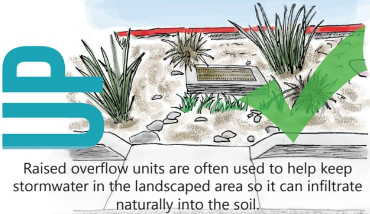
Raised overflow units are often used to help keep stormwater in the landscaped area so it can infiltrate naturally into the soil.
