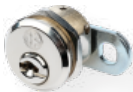
Cam cylinder no. 5558/30 RHM polished brass, nickel-plated, locking movement 90°, locking direction as desired, fitting dimension 25 mm
