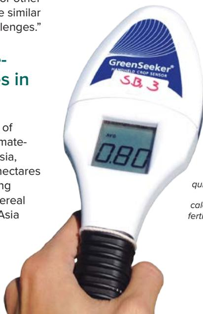
GreenSeeker is a compact sensor that quickly assesses crop vigor to calculate optimal fertilizer dosages.
