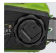
Guide bar tightening and adjustment
