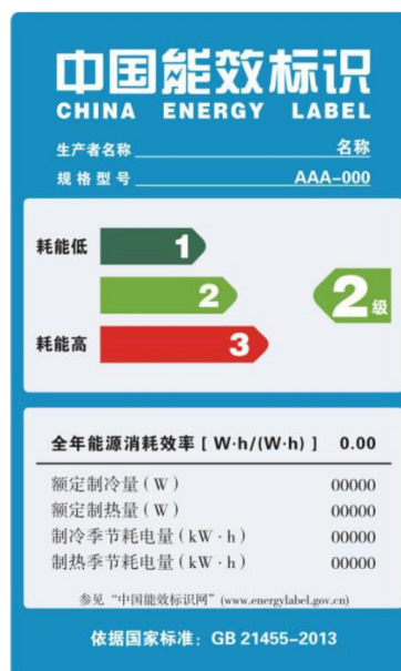
Figure 1: Example of the Chinese comparative Energy Label for variable speed air conditioners with both heating and cooling function
