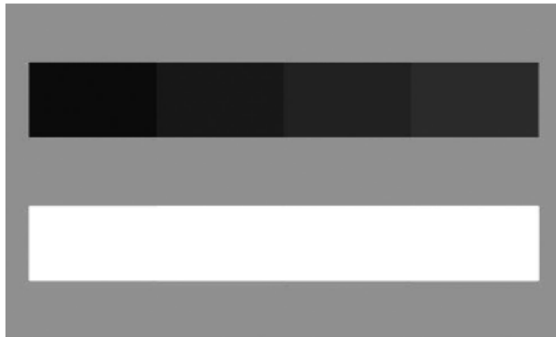
Figure 27: Eight-level gray pattern used in the Chinese TV test method
