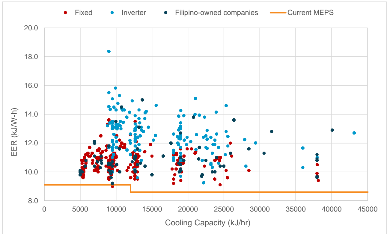
Figure 15: Cooling capacity vs. efficiency by compressor type ( N=3,096^{35} )
