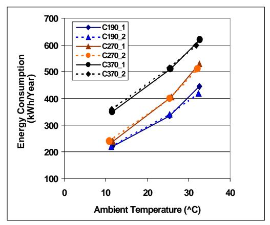
**Figure 1:** Annual energy consumption (kWh/year) with ambient temperature for AS/NZS for all-refrigerators (after Bansal<sup>13</sup>).
