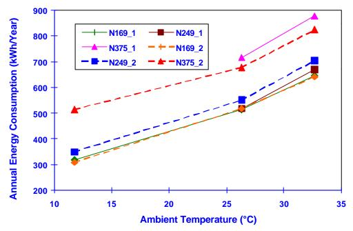
**Figure 2:** Annual energy consumption of different models of refrigerator-freezers with ambient air temperature - air relative humidity at 60% (after  $\text{Bansal}^{13}$ ).
