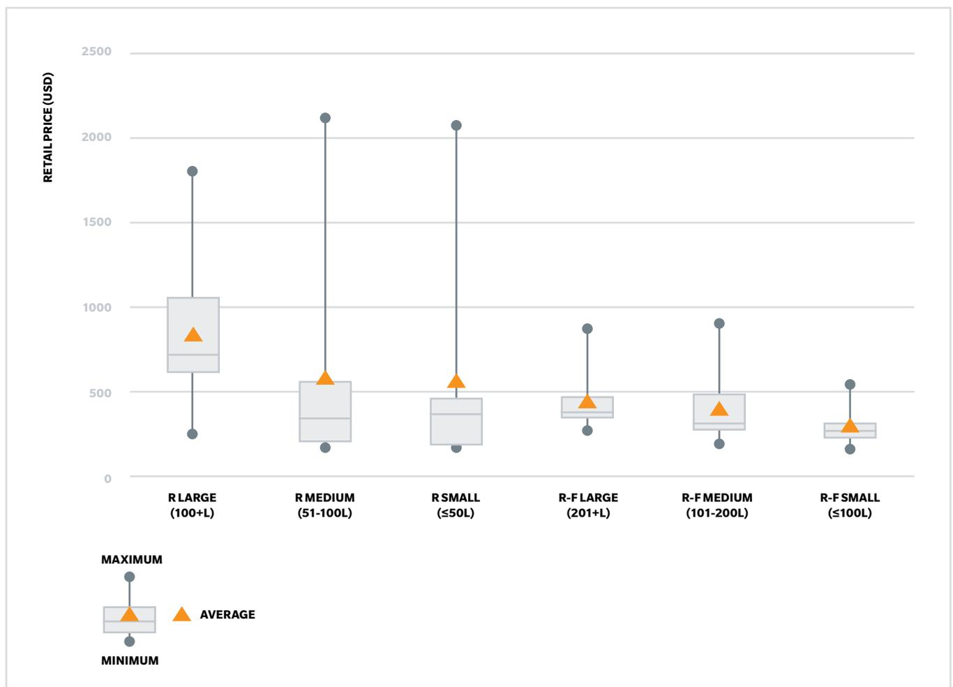
25. The refrigerators that have the highest retail price tend to be specialized off-grid refrigerators that are either designed to be used as a vaccine refrigerator, or use phase-change materials (PCMs)—a new cooling technology that uses water or other chemical substances to absorb and release thermal energy as its melting and freezing. Source: <https://docs.lib.purdue.edu/cgi/viewcontent.cgi?referer=https://www.google.com/&httpsredir=1&article=2043&context=iracc>.
