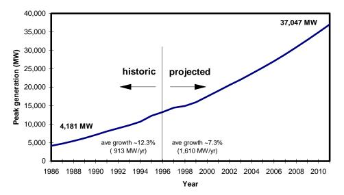
Figure 0.1. Historical and Forecast Generation Requirements for Thailand. In light of the recent economic slowdown, this is the most realistic available forecast of electric demand growth. It is based on the "very low-case scenario" in the 1996 Thai load forecast (TLFS 1996).
