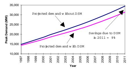
Figure 0.7. Projected Impact of DSM on Thailand's Peak Electricity Demand. (Source: World Bank 1996)
