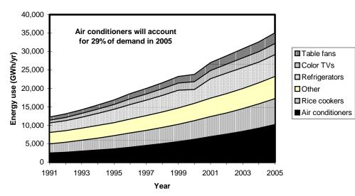
Figure 0.4. Forecast of Thailand Residential Electricity Demand by End Use. The end uses driving demand will be air conditioners (29% of demand in 2005), rice cookers (20%), and refrigerators (17%). Data from the most recent end-use forecast (TLFS 1993).
