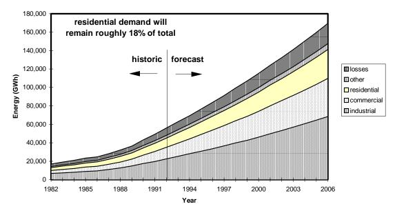
Figure 0.2. Thailand Electricity Generation Requirements by Sector. Based on latest available end-use data, in the 1993 Thailand load forecast (TLFS 1993).
