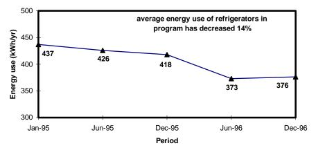
Figure 0.9. Average Energy Use of Refrigerators in Thai Labeling Program. (Source: DSM Office, EGAT)
