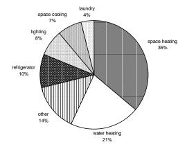
Figure Appendix A .3. U.S. Residential End-Use Breakdown, 1990. (Source: Lawrence Berkeley Laboratory)
