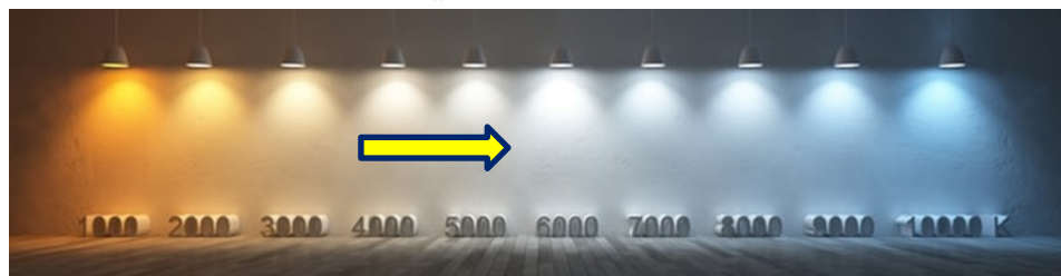
Figure 7. Movement along the curve in (a) results in changes in the CCT of white light in (b)
