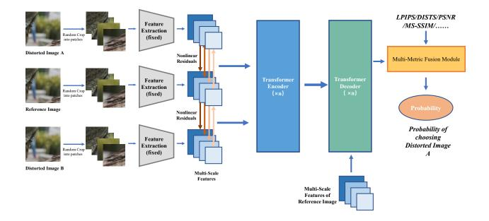
Figure 1. Overall architecture of the proposed image quality assessment method.
