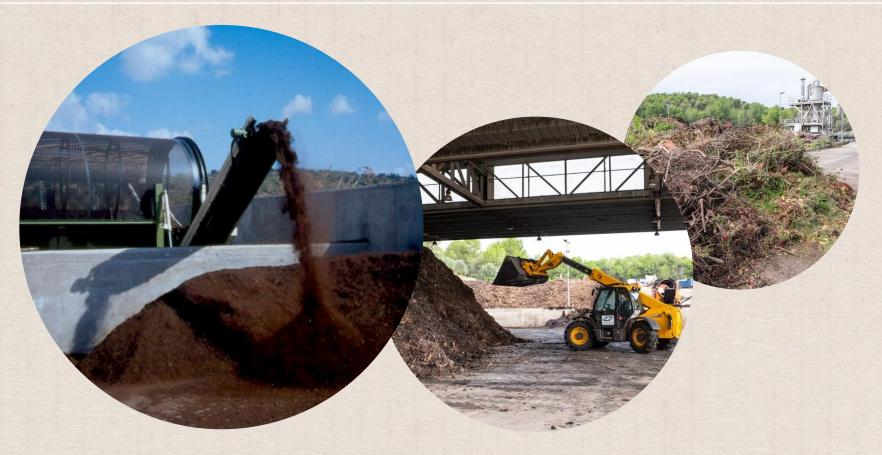
At our **compost plants**, we process organic waste (sludge, digestate and plant fraction) to produce compost which can then be used as a natural nutrient for crops.
