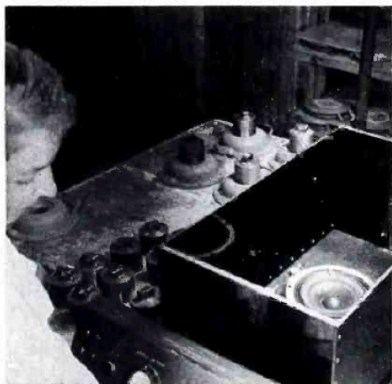
Magnetizing the speakers with a controlled pulse of energy produced in condenser discharge device.
