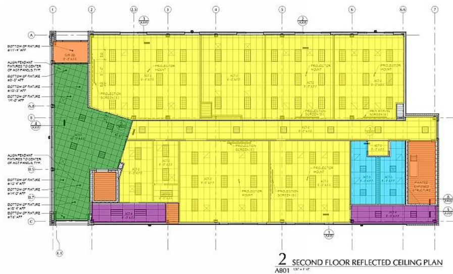
Figure 3. Reflected Ceiling Plan Takeoff Contractor
