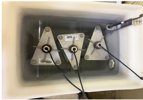
Figure 1. Equipment frame settings for CTE measurement
