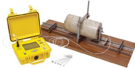
Figure 1. Emodometer setup for Young's modulus of elasticity measurement.
