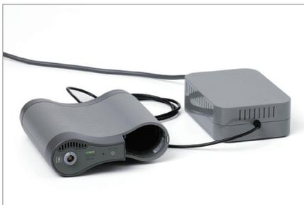
If you are switching batteries using the “No-Stop Swap,” always do so when the battery gauge light is yellow and **BEFORE** the “replace battery” alarm sounds. **IMPORTANT!** If the battery gauge light turns yellow and you are not near an outlet, you will need to power off the device before switching batteries.
