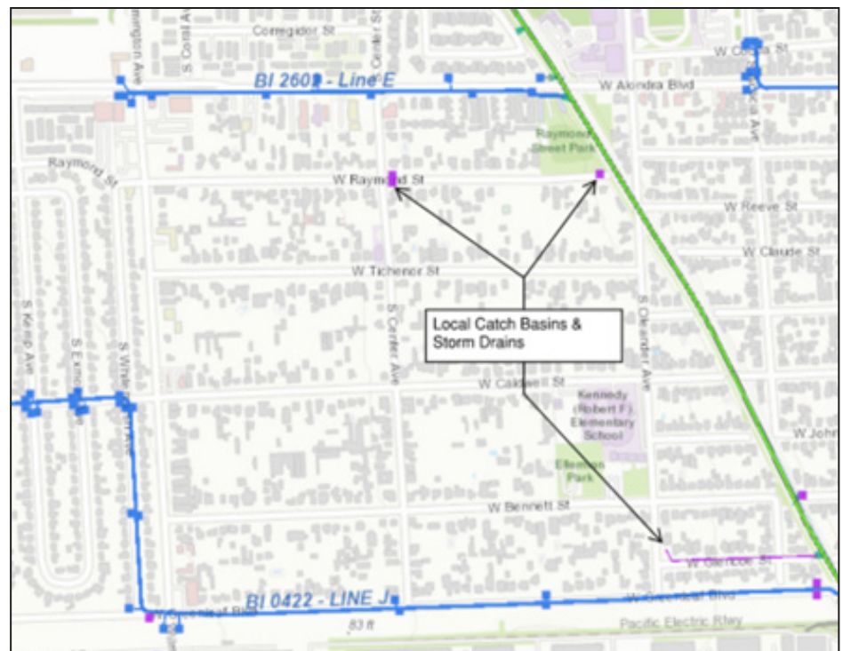
Figure 3. Local Storm Drains in Project Vicinity
