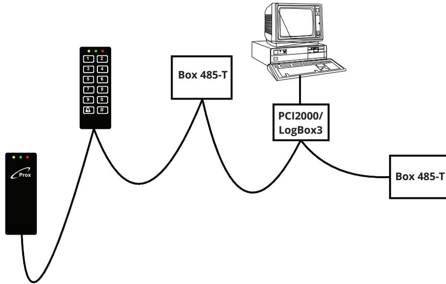
**Star connections must under no circumstances be used.** If this is the case with the 2000 system, the T connection are used, the T assembly must be **as short as possible**.
