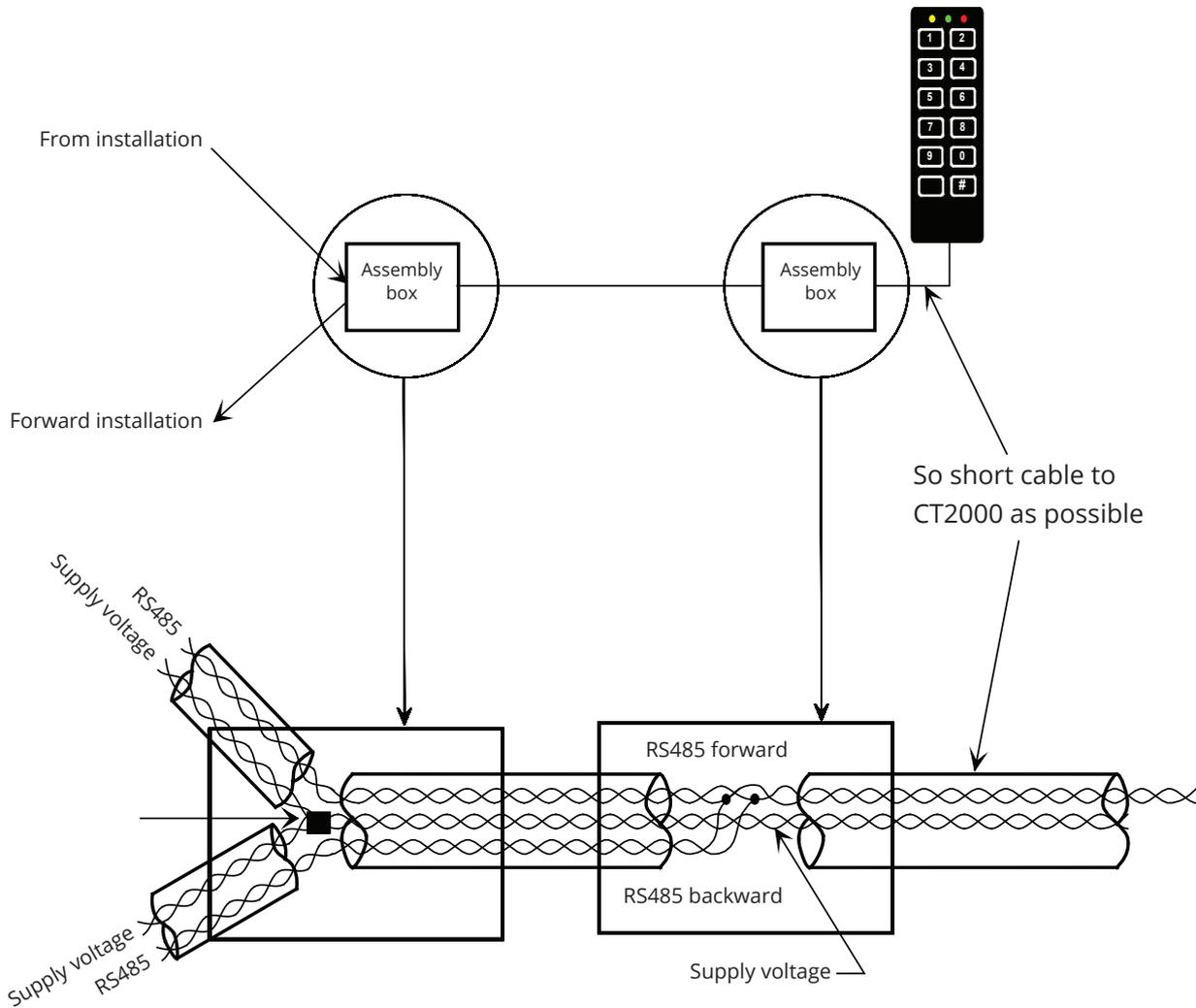
**Note** how the RS485 bus in separate pair of back and forth to the various units in the 2000 system. The power supply can freely be placed as it fits in the installation.
