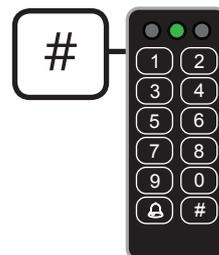
6. Key in < # > if you want to leave the programming mode. All 3 LED's will then illuminate shortly and the LED indicating the normal operating will illuminate (the yellow LED if the keypad has it's default programming).
