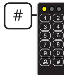
5. Repeat the touch on the < # > key (equals repeating programming "nothing" into the position). The green LED will illuminate. The value/code is now deleted.
