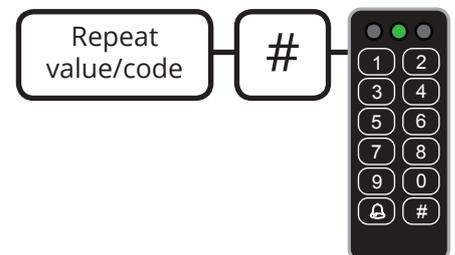
6. Key in < # > if you want to leave the programming mode. All 3 LED's will then illuminate shortly and the LED indicating the normal operating will illuminate (the yellow LED if the keypad has it's default programming).
