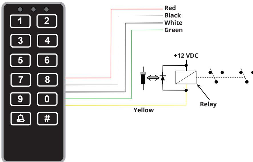
**Figure 6: Connection to a relay for general purposes.**
