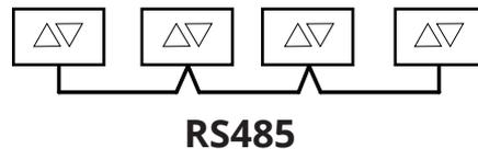
If the various units in the 2000 system each have their 12V DC power supply (230V AC connected to different phases), there may be a larger voltage difference between the devices, and RS485 circuits can be destroyed. To prevent this, it is necessary to make sure that the devices have the same potential.
