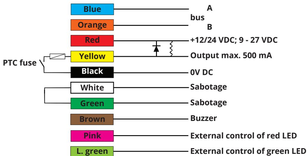
**The yellow core is the open collector, which gives a 0 VDC!**
