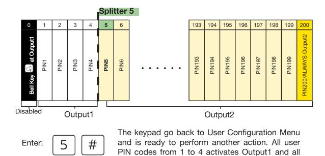
1 and 200 are considered "special values". If the Splitter value is 1, all user PIN's activates Output2, whereas if the Splitters value is 200, all user PIN's activates Output1. In both cases, the Bell Key function is used only to clear the PIN code buffer and doesn't activate Output1.
