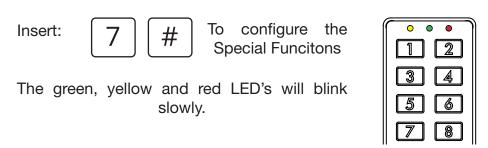
You can enable or disable the four special functions by pressing the corresponding key. The LED indicators will show whether a function is enabled (Green blinks) or disabled (Red blinks):
