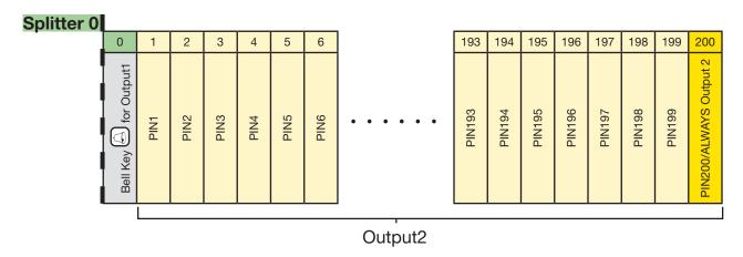
Note that if the configured value is **0** (default configuration), all User PIN codes activates Output2 and only the Bell Key , activates Output1.
