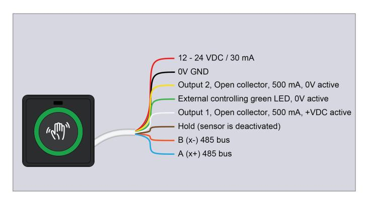
Also make sure that there is no object (protection stickers included) or any obstacles within 30 cm of the front panel to avoid any interference.
