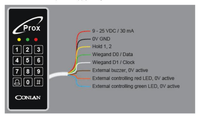
**Note:** Right after applying the voltage all LED's lights and the buzzer sounds, **do not** touch the reader untill the yellow LED is lit and the buzzer is silent.
