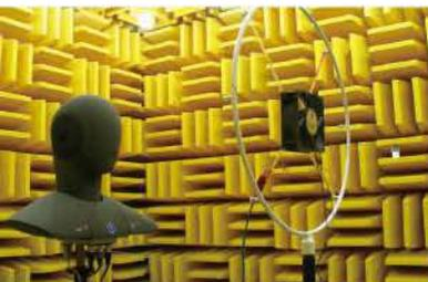
*Semi-Anechoic Chamber for Noise Test*
