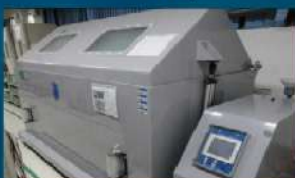
Salt fog test IEC 68-2-11
