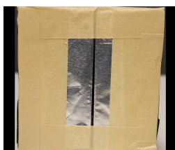
Slit between aluminum screens
