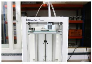
With the Ultimaker, designs can be tested before investing in tooling, which shrinks the percentage of required tool modifications from 30% to below 5%.
