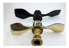
*Sylatech uses the Ultimaker to prototype sample parts for its customers, allowing them to test their designs without having to invest in tooling ahead of investment casting.*
