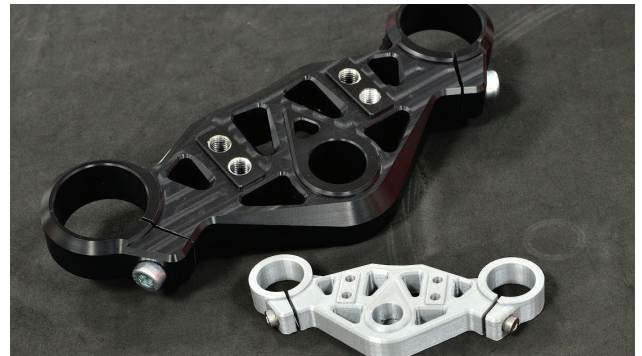
The capability to mount PLA prints directly onto motorcycles for thorough testing of tight tolerances and custom parts eliminates risk of design failure.
