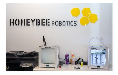
"When we are building a new type of robot, there's no point in getting metal parts when coming up with a new type of design because it is too expensive and takes too long. We'll print something that same day, put bearings, bushings, and other components into it, and then integrate a motor into it. This allows us to explore different parts of a robot that might be needed, and we can modify any design that does not work."
