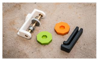
In the various phases of fabrication, it is often critical to inspect specific product features closely, or have the ability to view large parts on a smaller scale. 3D printing allows engineers to examine and adjust parts as necessary for more efficient production that reduces cost.
