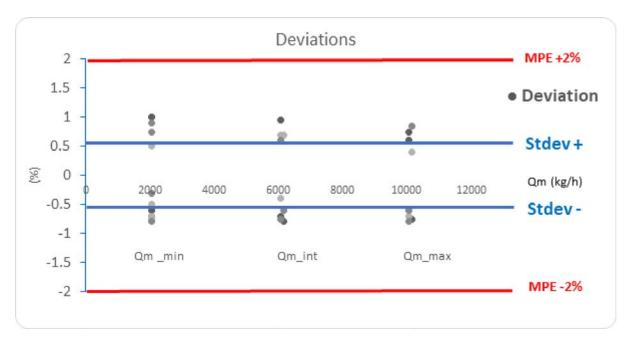
Standard deviation for these 30 totalisations:  $\sigma$  = 0.58 % If we apply the safety factor k=3, we get 3. $\sigma$  = 1.74 %: when referring to table 1, this system belongs to accuracy class 2 %. The accuracy class 1 % is out of reach.
