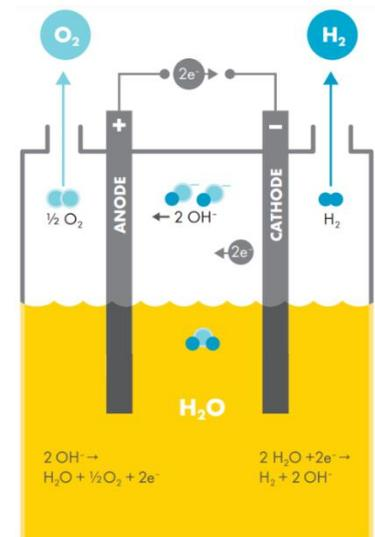
Figure 1: An electrolysis unit (Source: Shell Hydrogen Study)
