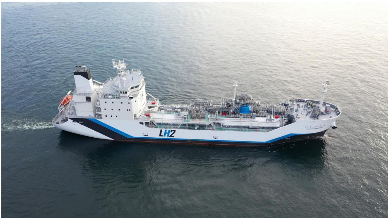
*The Suiso Frontier: the world's first liquefied hydrogen carrier. Image: HySTRA*
