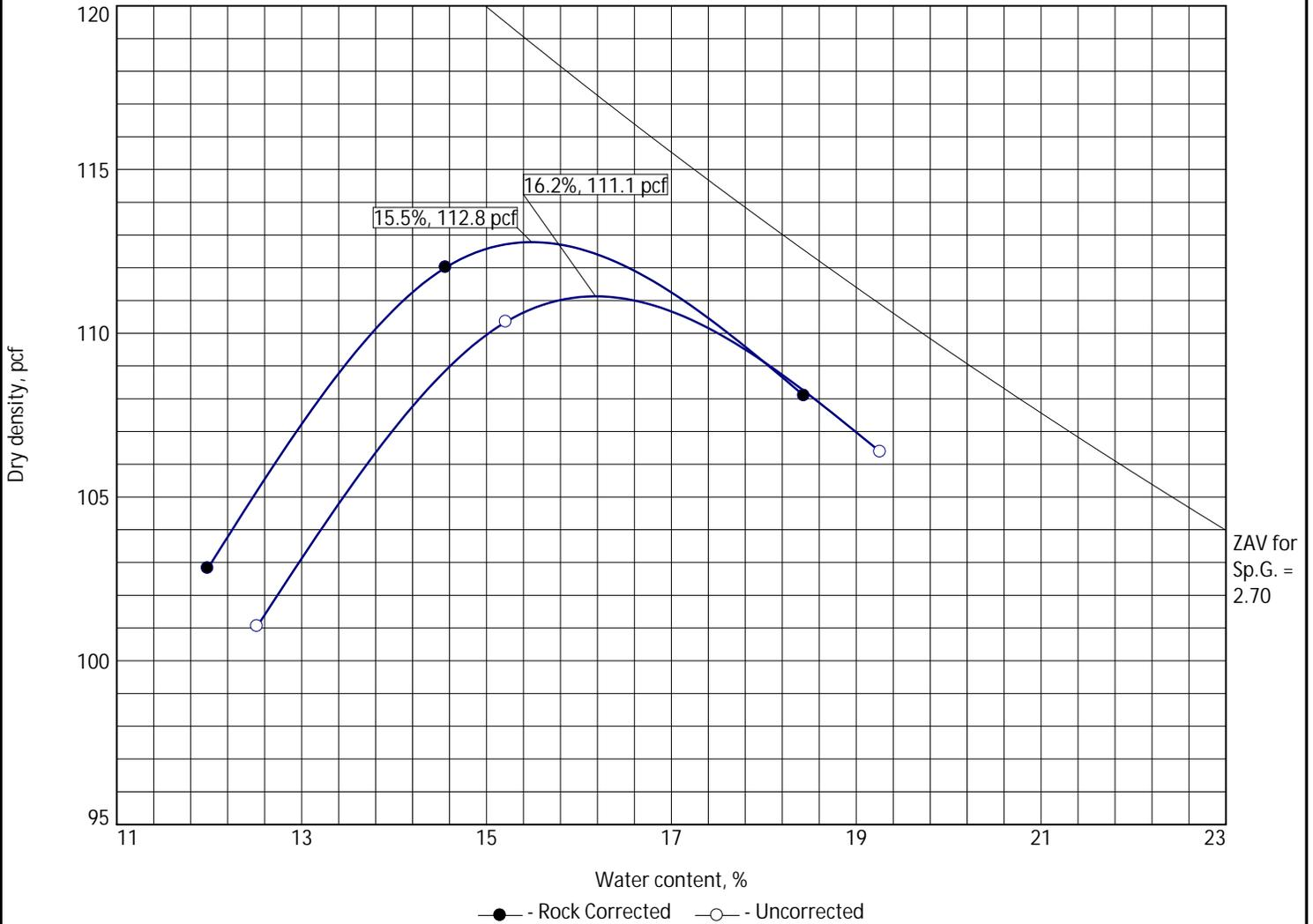
Test specification: ASTM D 698-12 Method B Standard
