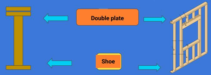
A *shoe*, also known as a single plate or bottom plate, is the bottom piece of the wall frame used to connect the wall to the floor or foundation.
