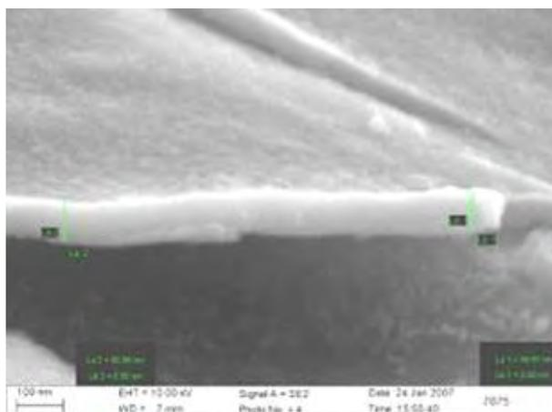
Fig. 10: SEM examination: fracture (7075)
