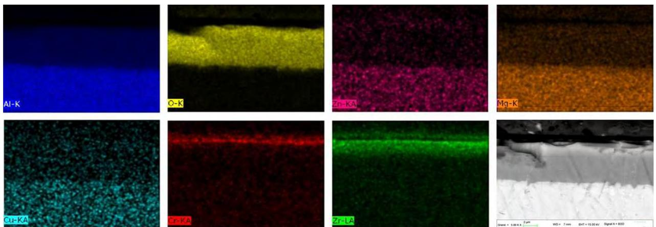
Fig. 8: SEM examination (back scattered electrons) of anodized 7175 T351 sealed with LANTHANE 613.3
