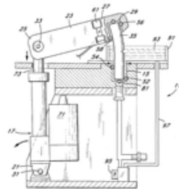
Fig. 1: RSL® Fig. 1: RSL® Loading Frame by Fracture Diagnostics Inc. as described in [1] (Image from US5585570)
