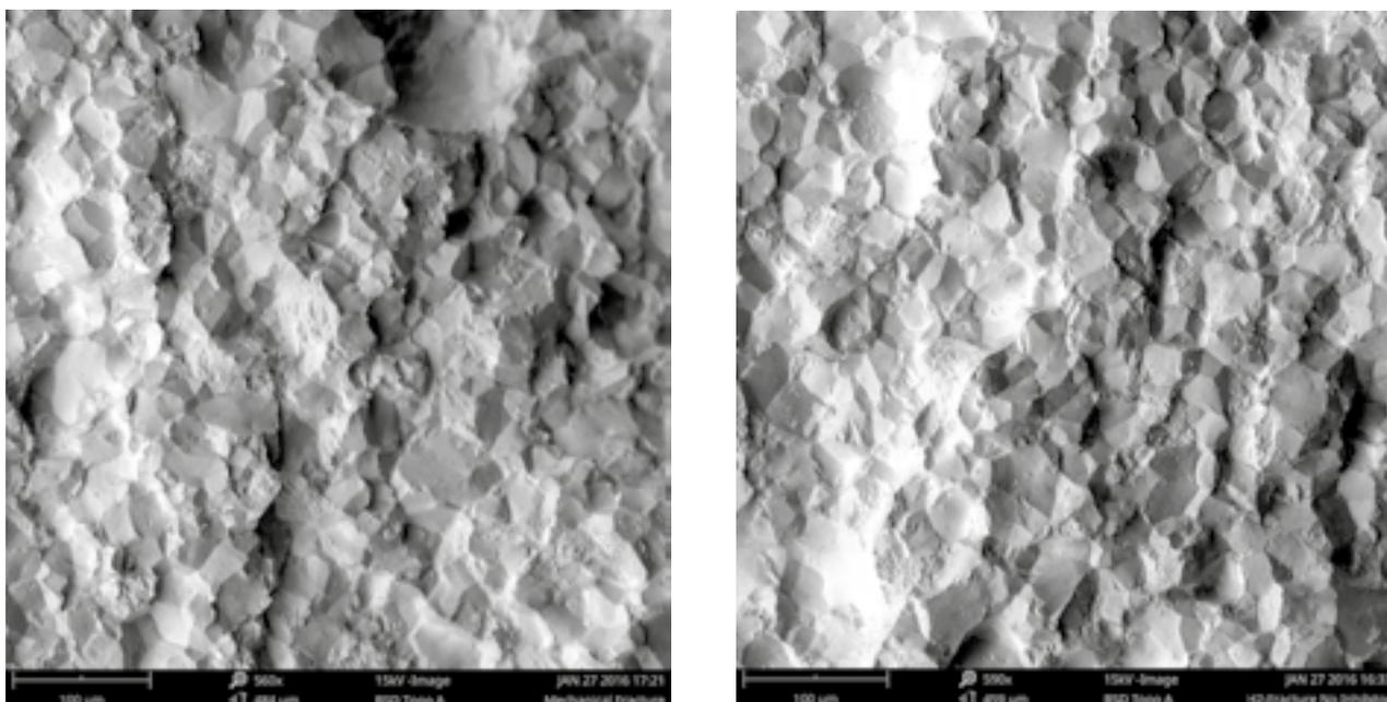
Fig. 4: SEM images of fractured surfaces of C-rings from a hydrogen induced fracture (right) vs. a mechanical fracture (left)
