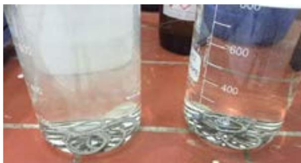
Fig. 2: Hydrogen evolution in a pickling solution without (left) and with (right) the addition of PICKLANE 50
