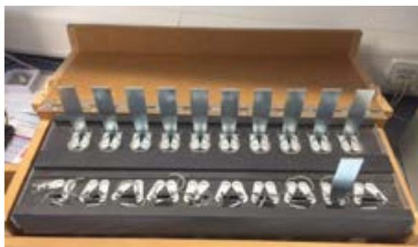
Fig. 3: Fractures after application of tensile stress to C-rings exposed to a pickling solution with (upper) and without (lower) the addition of PICKLANE 50
