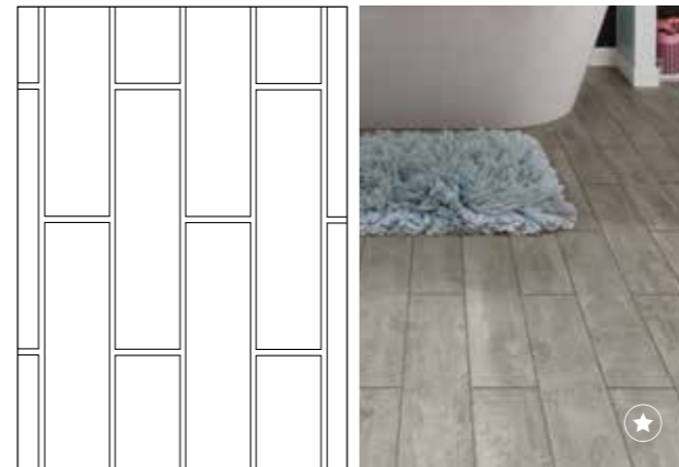
Slim tiles laid brickwork with surrounding strip. Design ref: 404
