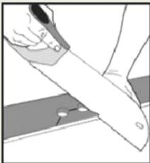
Installation at radiators. Drill the holes 20mm larger the diameter of the pipes. Cut out the panel (with the thinnest blade possible) as per diagram. Install the plank as per normal. Glue the cut out piece back again.
