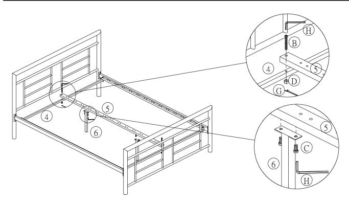
Step 4: Assemble the slats (7) as shown in the diagrams below and press the slat caps (F+E) firmly into the side rails (3) and the centre rail (5)
