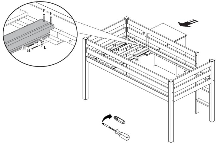
Next push the desk completely underneath the bed and attach the rear end of the fourth slat assembly with the final 2 screws (F). The desk should now move freely in and out on the wooden runners.
