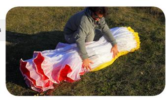
**Step 4.** Once the LE and TE of the wing have been sorted, turn the whole wing on its side.
