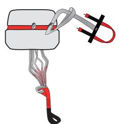
2 Tighten the handle/POD connection securely.
