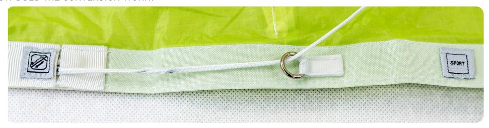
For the conversion to Sport-Mode the three middle top lines of the brake are lengthened and the remaining top lines shortened. A sophisticated system allows the conversion to be carried out by the pilot himself. You only need a rigid foil; the brake lines don't need to be untied. A detailed description for the conversion can be found in the PRO GUIDE and in the supplement included in the delivery.
