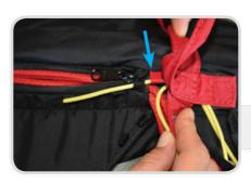
Now feed the yellow securing pins through the pin eyelets. Start with the pin located near the bridle. Each pin always starts with a red eyelet, feed the pin through each eyelet in order, make sure to not miss any inadvertently.
