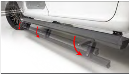
Powered step drops 8" when door opens and up to 15" below doorsill
