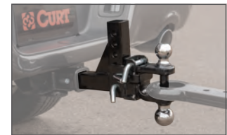
Welded trailer balls and removable clevis bar for lunette rings
