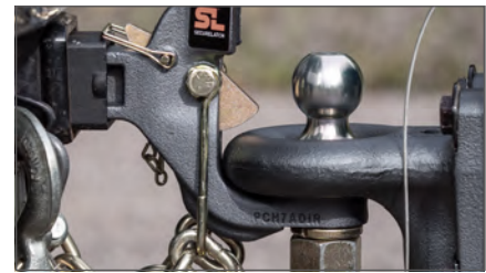
Cupped hook tightly holds lunette ring fore and aft to reduce chocking and noise
