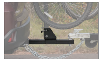
Towable shank allows use of the bike rack while towing a trailer
