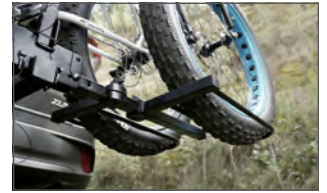
Designed to replace existing cradles on CURT tray-style racks
