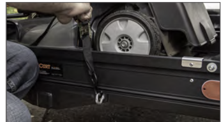
Six integrated eye bolts for secure attachment of straps or other tiedowns
