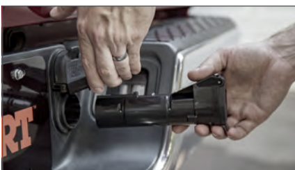
Insert Echo® between the vehicle and trailer
