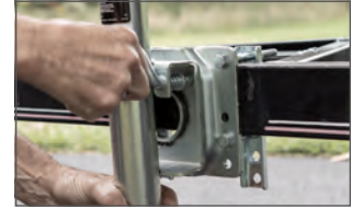
Heavy-duty pull-pin locks jack securely in place
