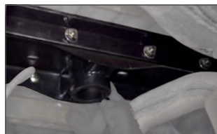
Step 2 - Bolt the install brackets and hitch to the vehicle frame
